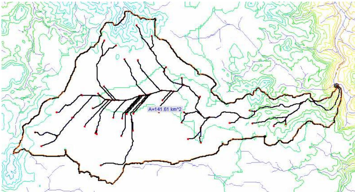
Figure 1 Initial WMS delineation derived using WMS
