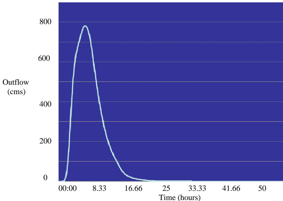
**Figure 4. Watershed runoff in a 20-year storm event and 85% ground saturation.**
